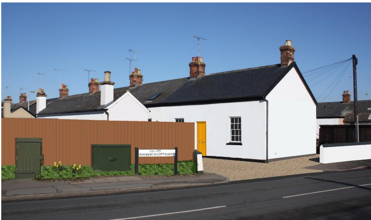
Fig. 47 – A mock-up of the entrance to the south row with a replacement fence, reinstated low boundary wall and new sash windows and front door to No. 116.
